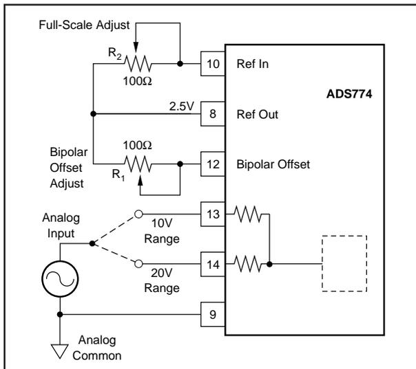
FIGURE 11. Bipolar Configuration.
