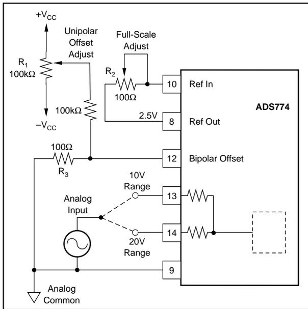
FIGURE 10. Unipolar Configuration.
